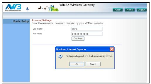
**3. Basic Setup Finished** – When the Basic Setup steps are completed the unit reboots and attempts to connect to the specified WiMAX network. Log in again to return to the Home page.
